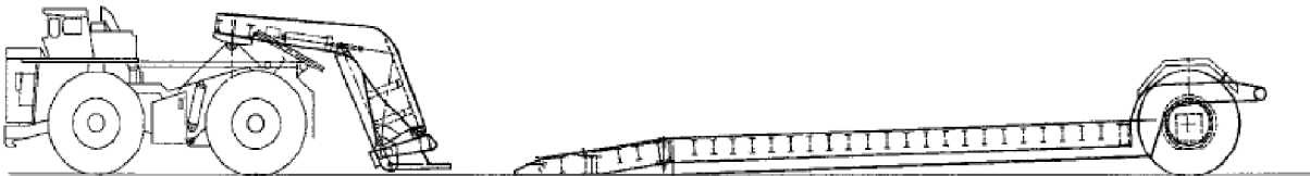
Rear Loading Design with Dual Rear Axle and Towing Attachment
